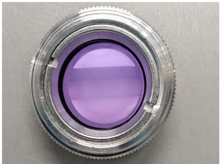
An RIE port showing generated plasma.
